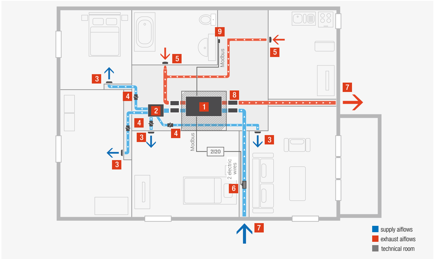
Typical apartment equipped with the DXR Unit, Reference version
